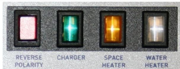
Red indicator, far left – Reverse polarity warning indicator. This illuminates when the green charger switch is turned on (see below) and the 230V supply polarity is reversed (see 3.10).
