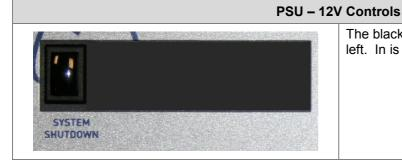
The black system shutdown button is shown on the left. In is ON and out is OFF.
