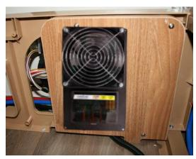
Plug the connectors (removed above) into the appropriate sockets on the rear of the VLM6. The connectors are colour coded and different sizes to prevent them being plugged in incorrectly. Ensure the retaining clips click into place after inserting each connector.
