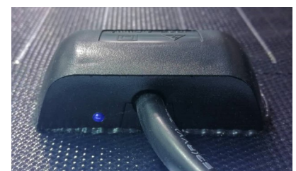
Junction Box with LED
